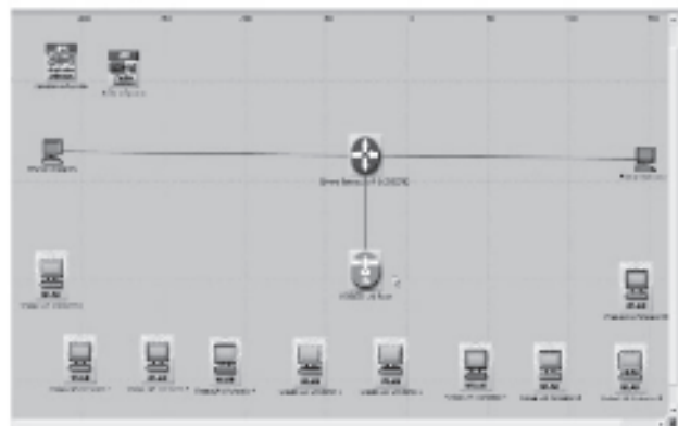
Figure 2: Simulation model of the Wireless LAN connected to the Ethernet which act as a gateway to the Internet
