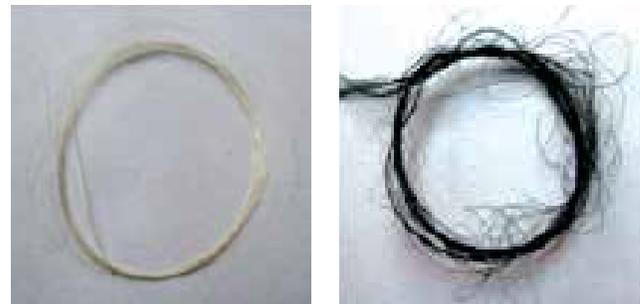
a) Before coating the original PEEK filament      b) After coating the black colored PEEK mono filament
