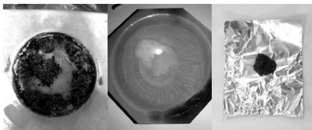
Figure 3: Synthesis steps a) mixing raw materials into deionized water, b) formation of sol, c) formation of gel, d) precursor xerogel, e) ground xerogel, f) annealed \text{BiFeO}_3 powder.
