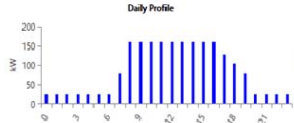
Figure 12: Typical daily profile (Residential Load)
