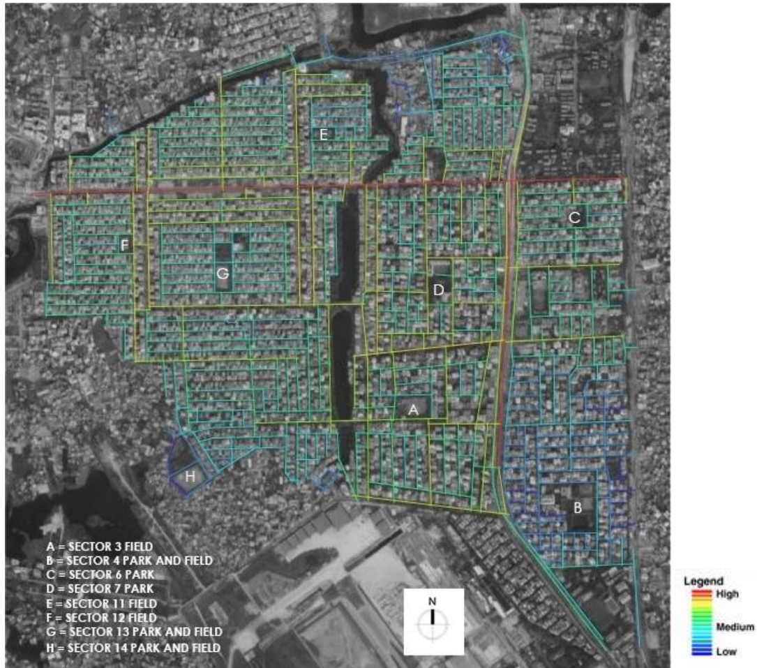
Figure 03: Juxtaposed Axial map of Uttara, showing the connectivity (CN) and location of parks and fields
