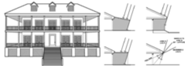
Figure 16:Passive Cooling System,Basc.Pnnl.Gov/Resource-Guides[1]
