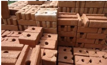
Fig 54:CEB Blocks, source https://www.structuralguide.com/compressed-earth-block/ [26]
