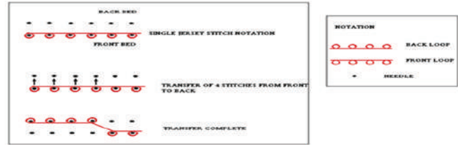
Figure 7 . Loop transfer on V-bed knitting machine [12].
