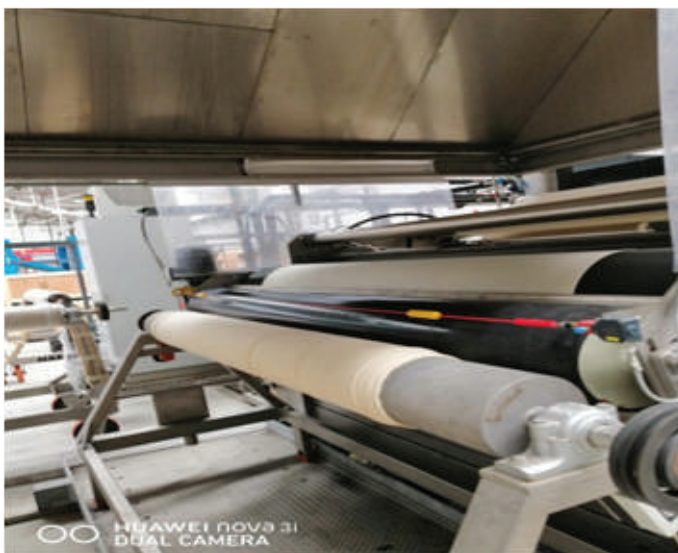
Figure 1. Nano-dye Machine for pretreatment of cotton fabric.
